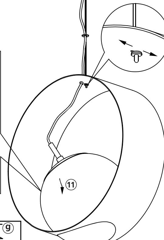
If the metal shade is not level, adjust the position of the steel wire.
