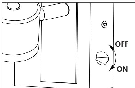
If the fixture doesn't light, check switch on fixture to make sure it is turned on.
