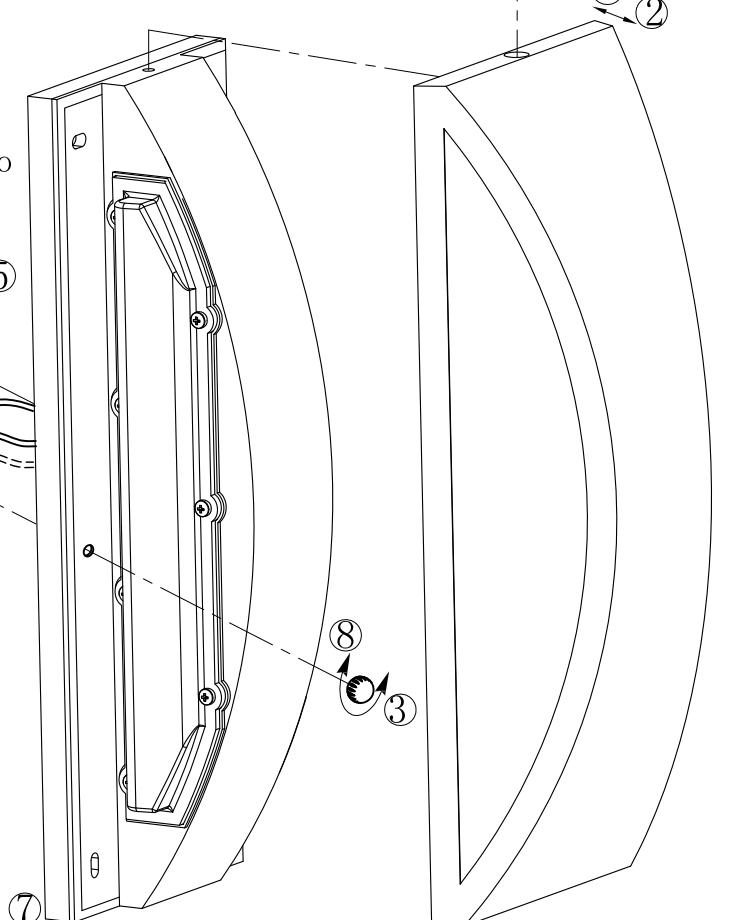
Mount fixture in vertical position only with drain hole at bottom
