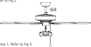
3. Attach the light kit to the switch housing using the 3 screws removed in step 1. Refer to Fig 3.
