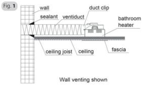
Locate a position for the exterior vent on the wall not more than 3.0 m from the unit, 4. and allows the ducting to remain straight. (Refer Fig. 1)
