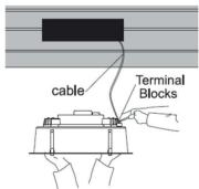
Open the terminal block cover on the housing and make connections as per wiring 12. diagram and reattach the terminal block cover. (Refer Fig. 3)
