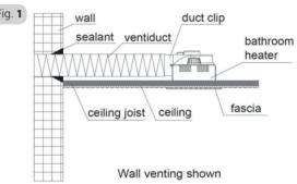
Locate a position for the exterior vent on the wall not more than 3.0 m from the unit, and allows the ducting to remain straight. (Refer Fig. 1)
