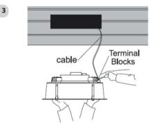
12. Open the terminal block cover on the housing and make connections as per wiring diagram and reattach the terminal block cover. (Refer Fig. 3)
