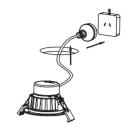
Insert the plug into the power socket located in the ceiling. Please note if a series and the ceiling. ceiling. Please note, if no power socket is present, one will need to be installed by a licenced electrician.
